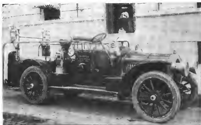
THOMAS FLYER CONVERTED INTO FIRE ENGINE BY A. C. WEBB.
